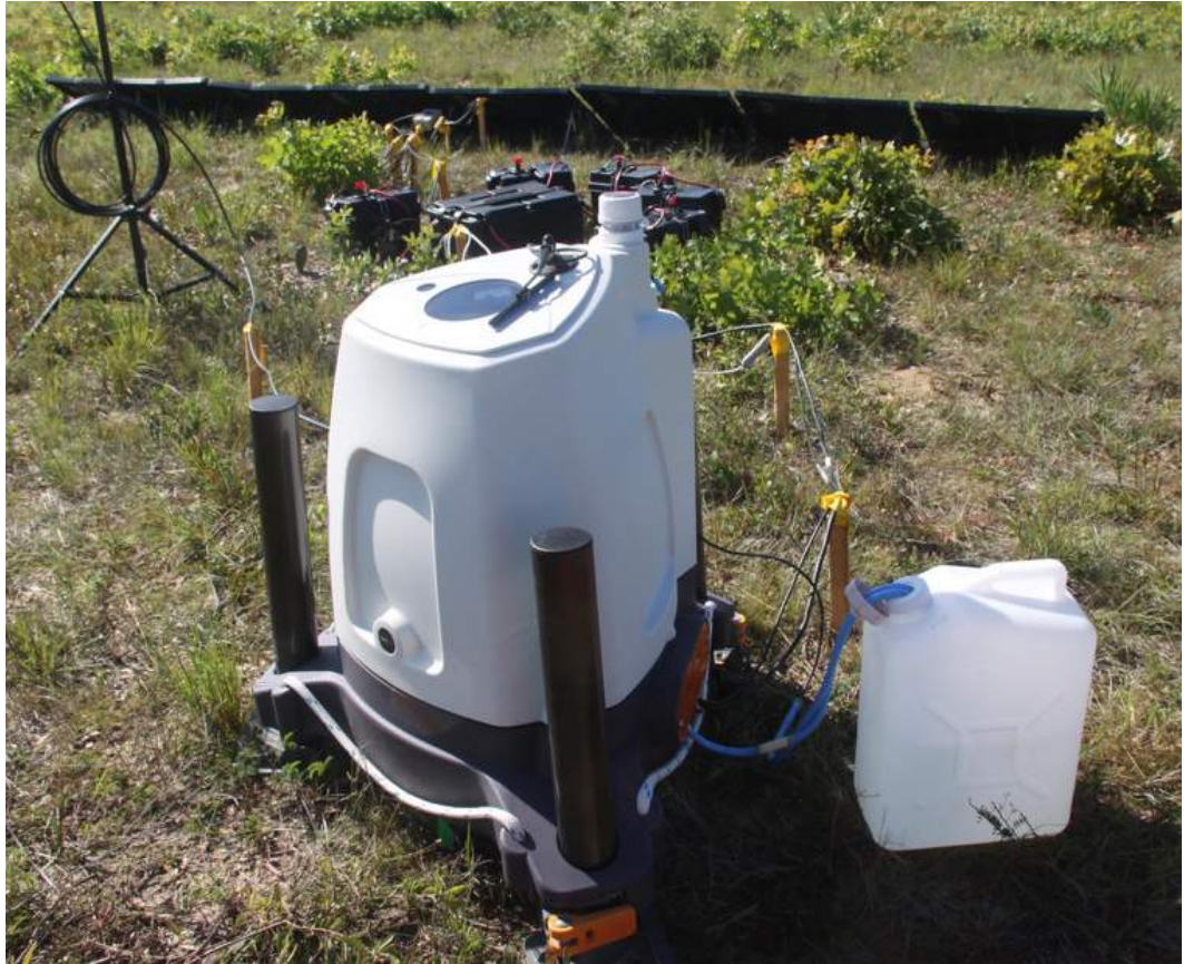
Figure 10: LIDAR wind measurement system.
