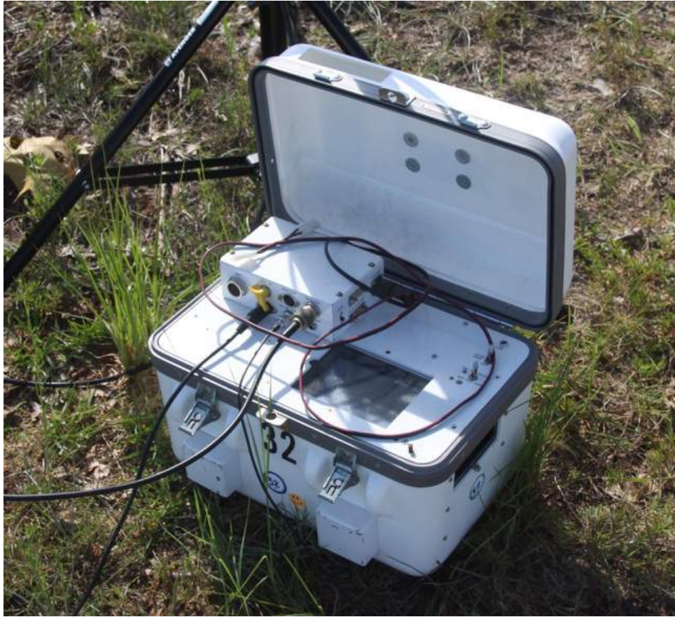
Figure 6: Wireless Acoustic Measurement System.
