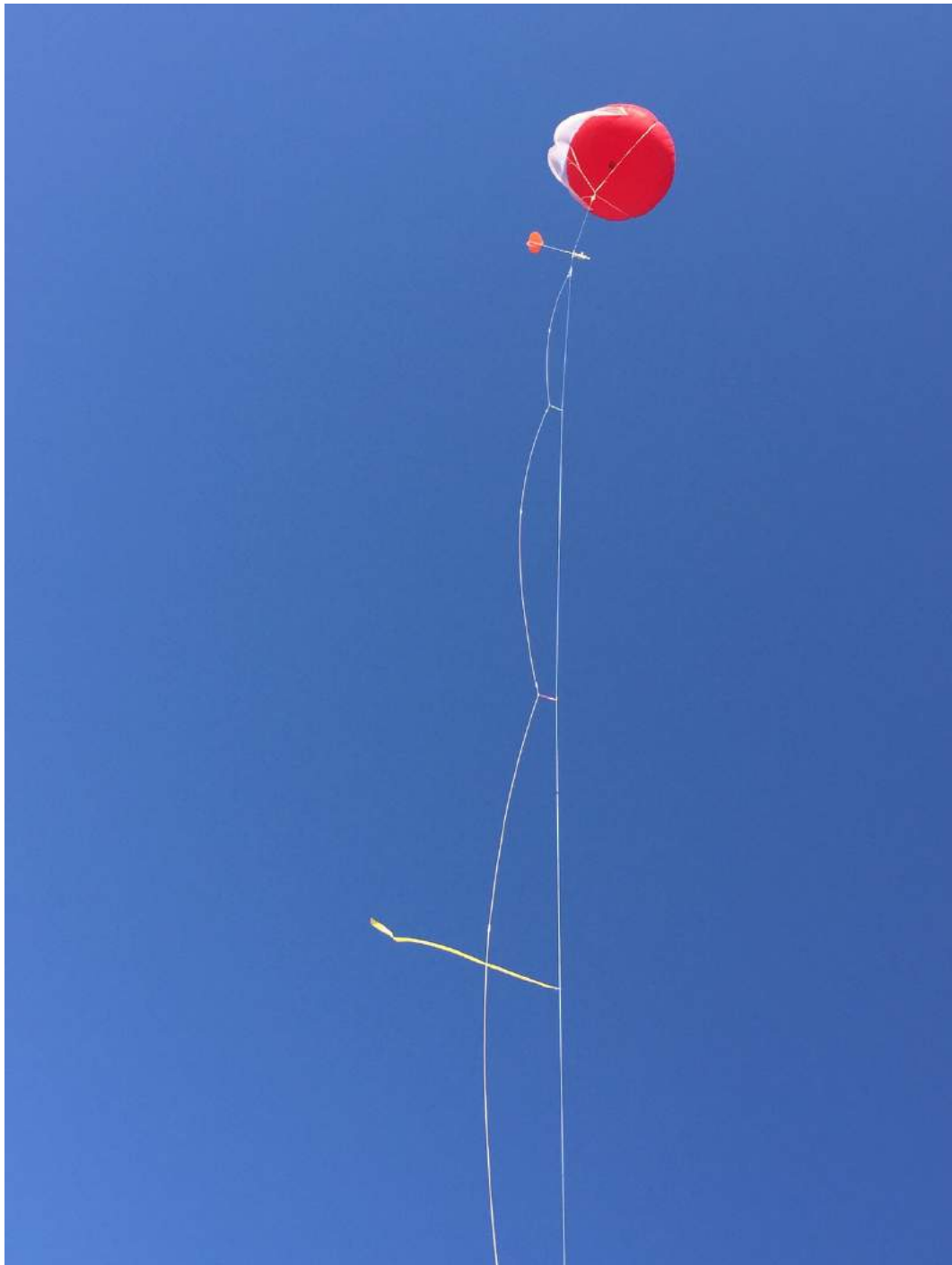
Figure 9: Temperature string attached to weather balloon.
