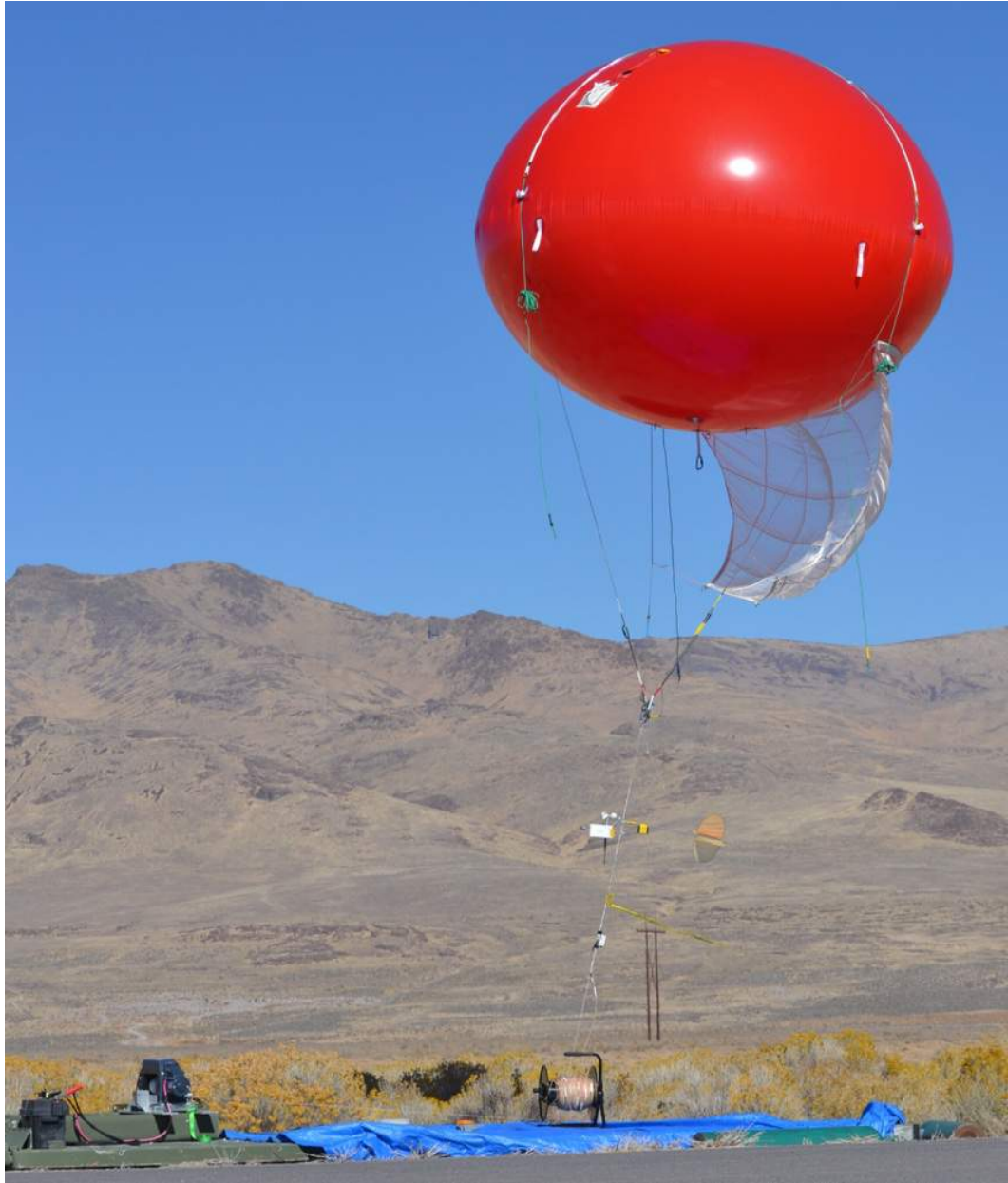
Figure 8: Tethered balloon weather system.
