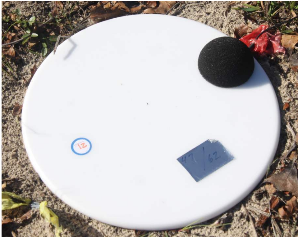
Figure 5: G.R.A.S. 67AX flush mounted microphone.
